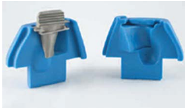
Masking for Grit Blasting, Triton / Stratasys / AFRL SBIR
