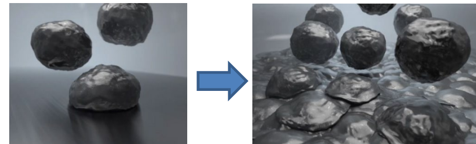
Rendered time lapse (left to right) of cold spray particle "splat" metallurgical bonding
