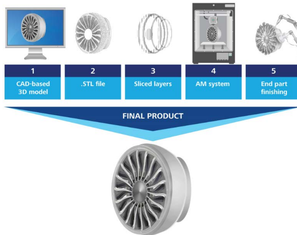
Figure 1. Additive manufacturing (AM) process flow
